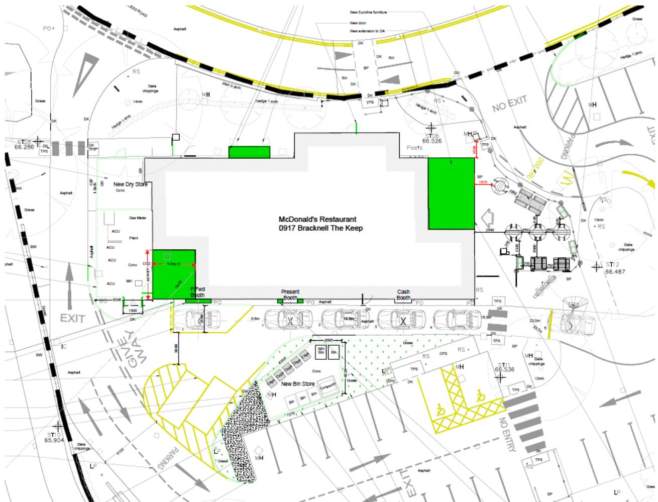
5.2 The extensions would be to the front, side and rear of the building. The front extension would project 1.1m forward of the building with a width of 3.82m, forming an enlargement to the female WC. The side element would be an infill extension with a width of 4.34m and a depth of 6.75m, forming an enlargement to the restaurant area.
